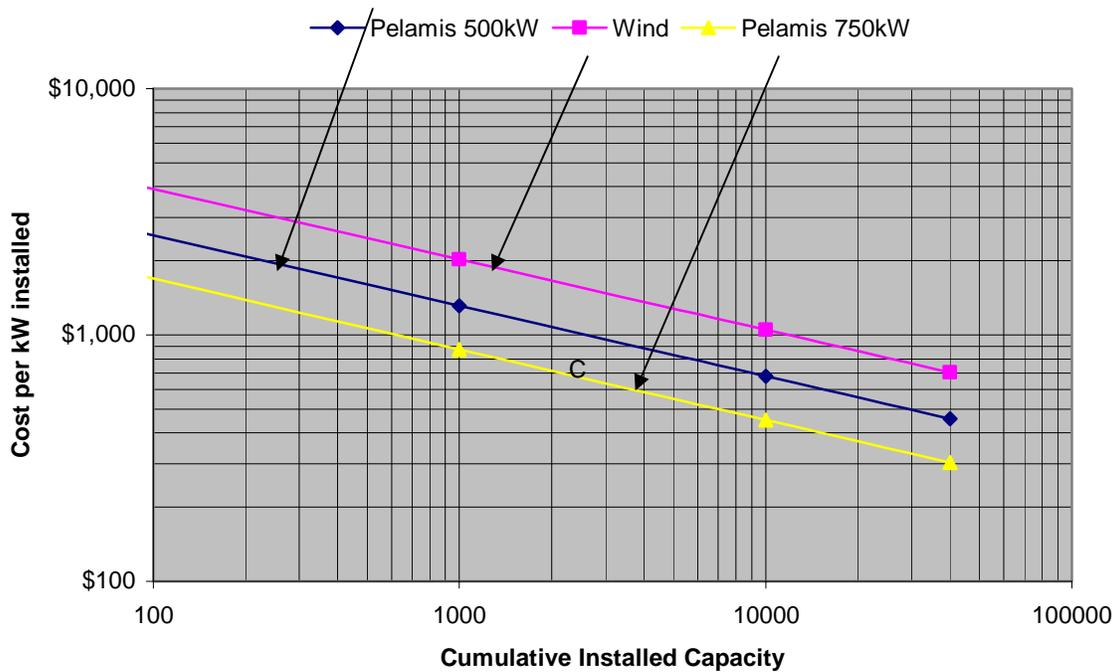
**Figure 25: Installed Cost per kW installed as a Function of Installed Capacity**
