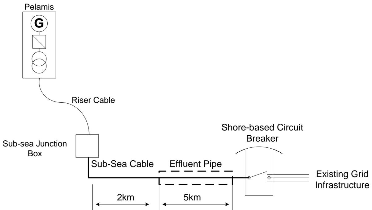
**Figure 15: Electrical Interconnection of a 1 Pelamis Pilot Plant**
