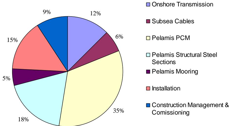
**Figure 18: Pie Chart of cost centers for single unit installation**
