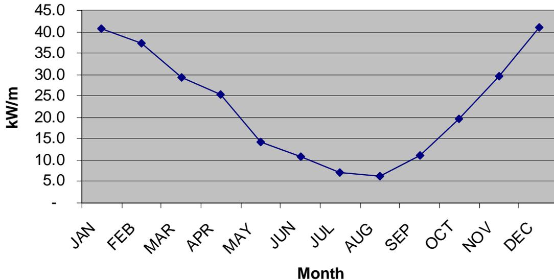
**Figure 3: Monthly Average Wave Power Flux (kW/m)**
