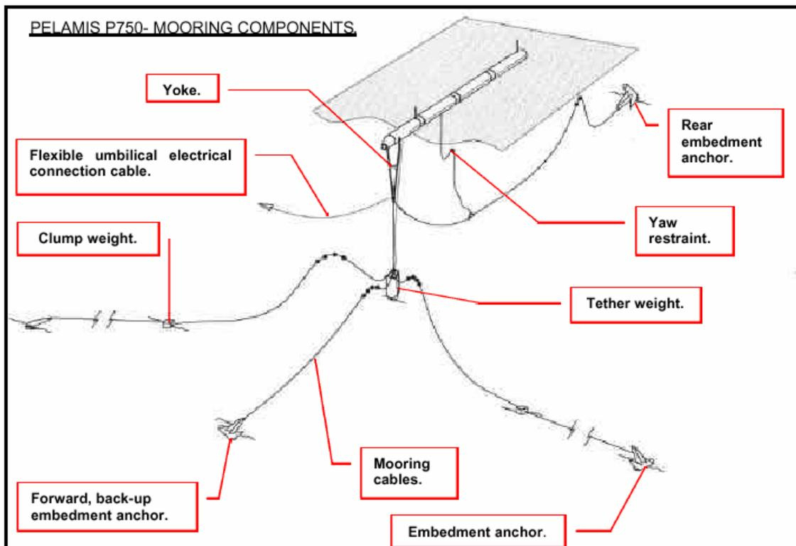
**Figure 9: Mooring Arrangement of Pelamis**
