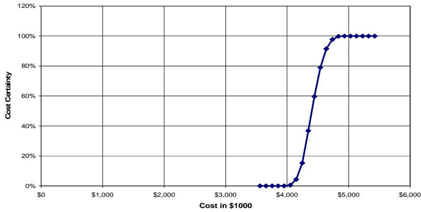
Figure 19: Installed Cost Uncertainty based on Monte Carlo Simulation
