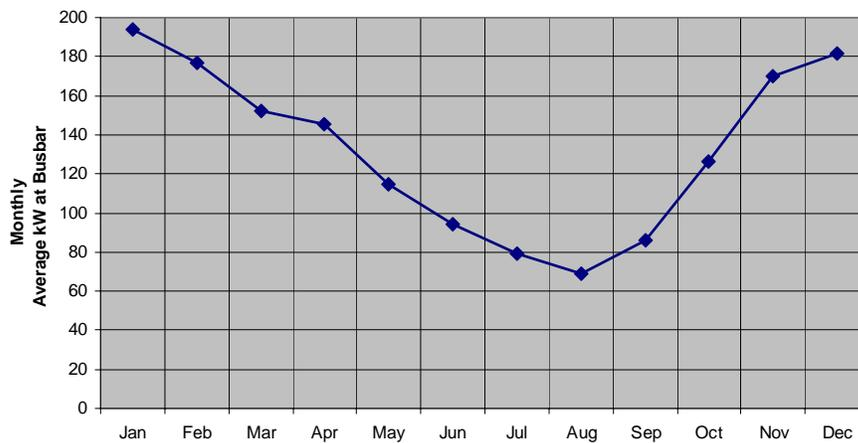
**Figure 17: Monthly average power delivered to bus bar – Pilot Plant**
