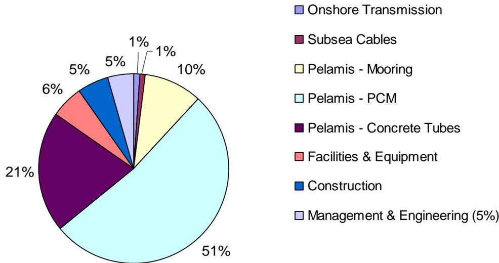
**Figure 20: Installed Cost Breakdown for commercial scale plant**
