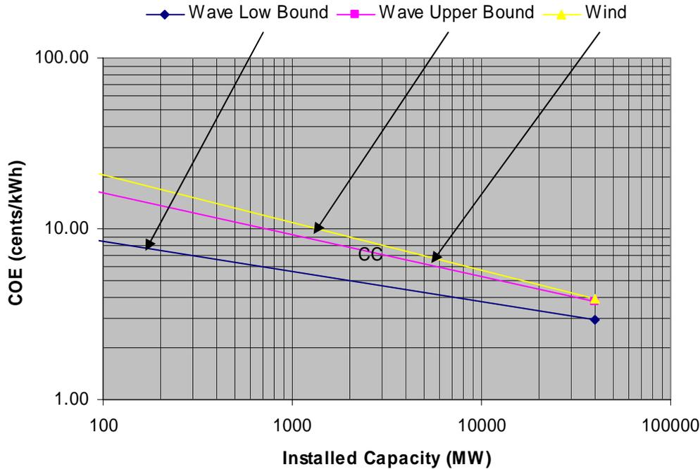
**Figure 26: Levelized COE comparison to wind**
