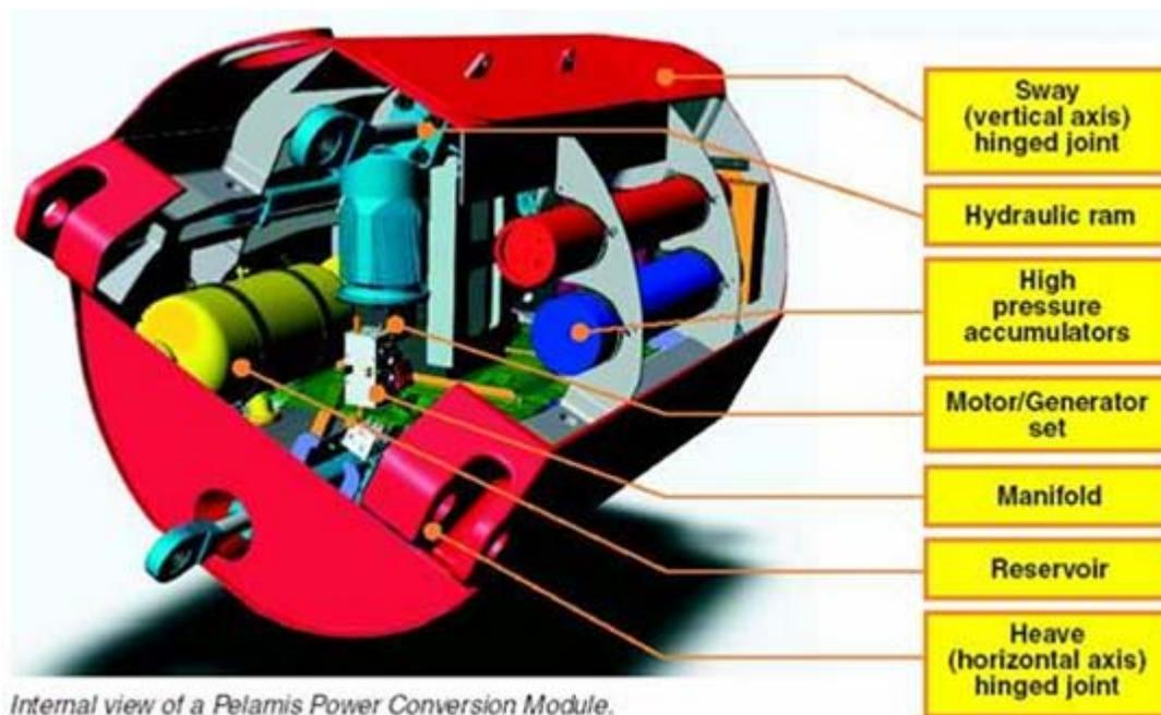
**Figure 7: Internal View of the Pelamis PCM**
