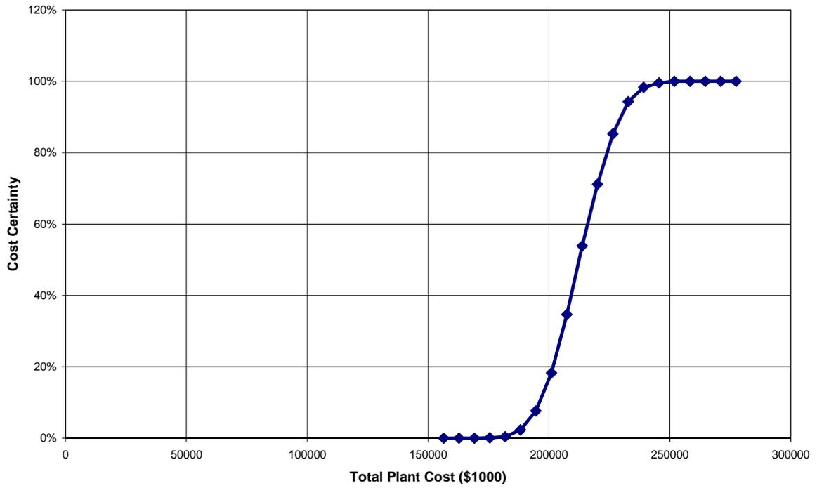
Figure 21: Installed Cost uncertainty S-curve
