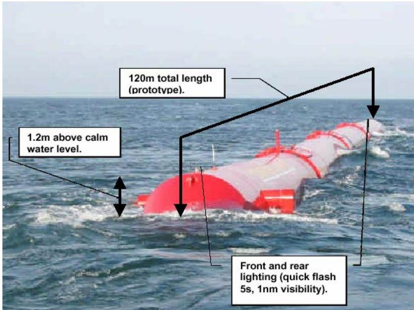
Figure 4: Pelamis pre-production prototype undergoing sea-trials
