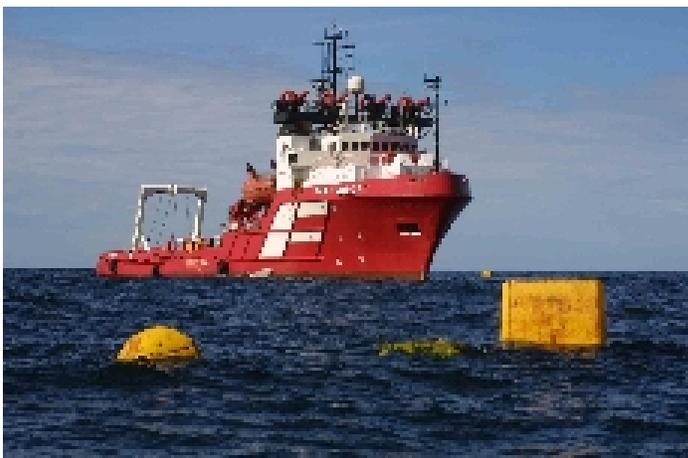
**Figure 13: AHATS class vessel used for prototype installation in UK**
