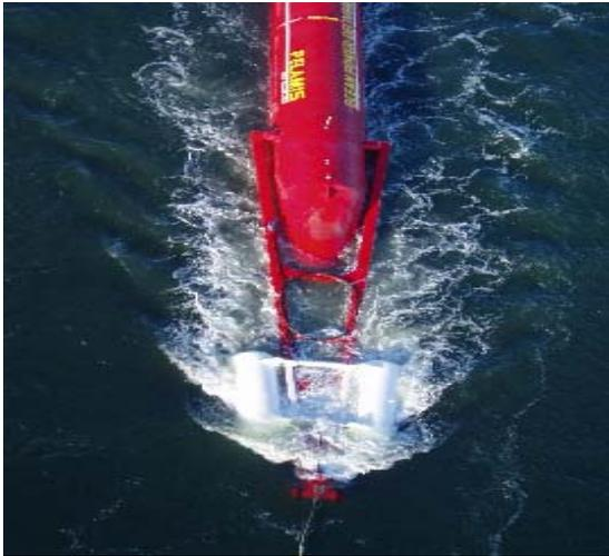
**Figure 14: Towing the Pelamis P-750**
